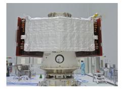
Both modules, MTM and the mini stack (MPO/MMO) have been installed on their dedicated fuelling stands inside the S5B cleanroom. Dry mass weighting of the modules and the fuelling setup has been completed.
