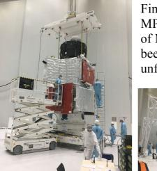
Final mating of the "mini stack" (MMO integrated on MPO) together with MTM will be performed after fuelling of MPO and MTM. In order to reduce risk, the mating has been successfully exercised inside the clean room with the unfuelled modules.
