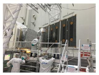
After SA integration on MPO, the SA has been folded, followed by the release for deployment verification. After successful deployment the MPO SA wing has been finally folded for flight.
