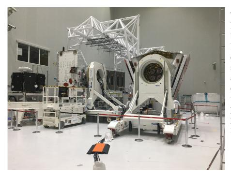
Today the electrical MCS configuration has been restablished with MPO next to SA deployment rig. This setup allows MPO MLI activities and MCS count down rehearsal test being performed in parallel to avoid a potential schedule impact.
