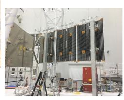
In parallel to the MCS test activities, the MPO SA has been unpacked and deployed inside the deployment rig. Visual inspection is on going.
