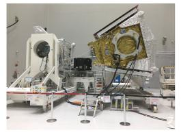
BepiColombo is in electrical stack configuration. The three modules MMO, MPO and MTM are located close together, connected via extention cables. The Abbreviated Functional Test (AFT) of the Mercury Composite Stack (MCS) configuration has been successfully completed on both redundant sides.
