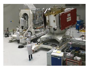
Today, the 3 modules have been rearranged inside the clean room, and the electrical MCS configuration has been achieved using extension cables. The test setup is ready for next week functional verification.
