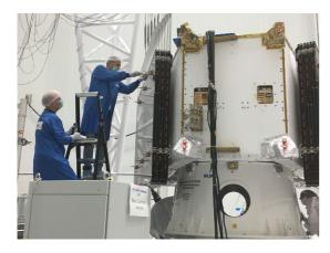
Following the successful validation of the +X SA, the array has been positioned, aligned and mechanically and electrically integrated on MTM. Electrical checks and illumination test have been completed. After folding the +X SA wing, the final deployment test has been successfully performed. Final wing folding into launch configuration has been completed, and the red-tag protection cover was mounted. MTM is ready for next week MCS test.
