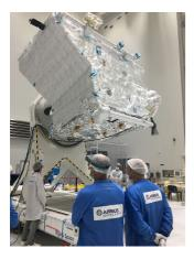
MPO MLI integration around the Antenna Pointing Mechanism (APM) for the High Gain Antenna (HGA) and Medium Gain Antenna (MGA) was started. Low temperature MLI integration on +Y panel has been completed. Glow test of the MPO Solar Array (SA) Thermal Knife (THK) was successfully performed. Periodic environment radiation measurements close to SIXS/MIXS performed, no anomaly found.
