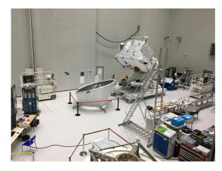
MPO OBC software has been successfully loaded and validated. MLI activities are on going. S/C has been positioned in two different orientations for reaction wheel maintenance, which has been completed as well.
