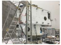
MTM drying of Xe tanks is on going. Xe loading equipment setup and connection has been completed inside the clean room. MLI integration/sewing is on going in parallel on MTM.
