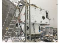
MTM drying of Xe tanks is on going. Xe loading equipment setup and connection has been completed inside the clean room. MLI integration/sewing is on going in parallel on MTM.
