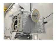
On MPO, +X and -X side panel MLI integration and sewing has been completed. 5N- and 22N- thrusters were inspected and cleaned, the leak check is on going. Blast shields have been located around MPO as
