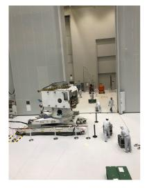
Most impressive activities during this week, was the build up of the solar array deployment rig and the start of the related alignment tasks, which required logistical effort in re-arranging the clean room layout in order to minimize the impact on the three module activities
