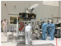
Intensive electrical checks of MTM PCDU integration have demonstrated full functionality. In parallel, MPO alignment verification was completed. Finally MCC3 (Multiple power point Conditioning Circuit) has been integrated on MPO. MTM and MPO have been located next to each other, and both modules have been connected similar to the MCS electrical stack. This configuration was needed to validate MCC3 functionality, which has been successfully completed.
